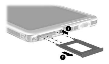
Removing the PC Card Device
